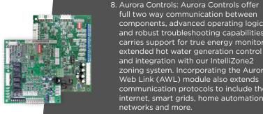
full two way communication between components, advanced operating logic and robust troubleshooting capabilities. It carries support for true energy monitoring, extended hot water generation control and integration with our IntelliZone2 zoning system. Incorporating the Aurora Web Link (AWL) module also extends communication protocols to include the internet, smart grids, home automation networks and more.
